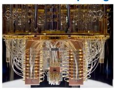
RF transmission lines are a critical path for both steering and data collection of Qubit information; coaxial assemblies must be phase stable, non-magnetic, and built for extreme temperatures.
