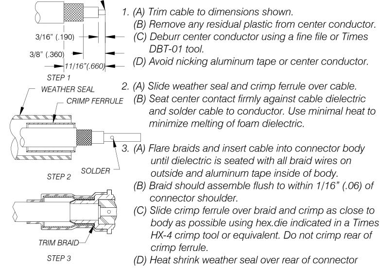
body and down on to cable jacket using hot air gun.
