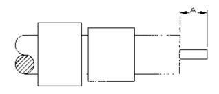
STEP 5. Install contect,  $C = 0.020^{\circ}$ Solder on the contect using 60/40 solder. Feed solder thru solder hole while heating the contect. Trim braids to dimension  $X = 0.400^{\circ}$
