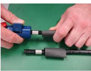
3. Debur the center conductor using the debur tool on side #2 of the CST-400 or a file. Make sure that the center conductor is free of plastic film.
