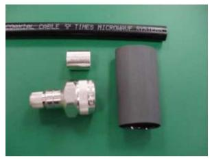
2. Slide the heat shrink boot over the end of the cable, followed by the ferrule. Slide End 1 of the CST-400 prep/strip tool over the end of the cable. Rotate the tool in a clockwise motion while pressing down on the blade cartridge. Spin the tool until you have made a full revolution with the button fully depressed. Remove the tool and purge the plastic pellet.
