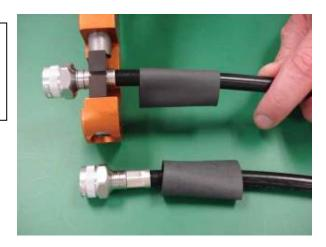
7. Slide the boot up to the back of the coupling nut and shrink with a heat gun until a lip of adhesive can be seen at both ends of the boot.
