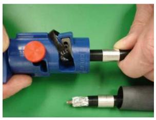
5. Place the connector over the outer conductor of the cable. Push and turn the connector onto the cable until it is fully seated. Bring the ferrule all the way up to the back of the connector.
