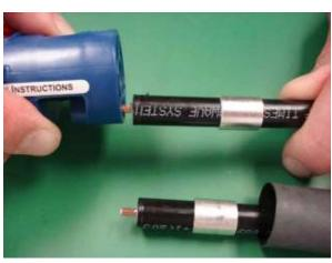
4. Make sure that the thumb wheel is set for "crimp". Insert the cable into side #2 of the CST-400 prep/strip tool and rotate the tool in a clockwise motion until the tool spins freely. Remove the tool (If you are using a knife to accomplish this step, be careful not to nick the braids).
