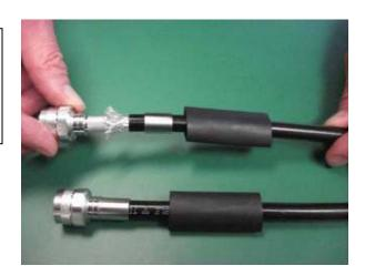
6. Use a CT-300/400 (0.429" hex) or equivalent crimp tool to crimp the ferrule once directly behind the connector. DO NOT DOUBLE CRIMP.
