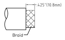
1. Cut the cable squarely and cleanly using the CCT-01 cutting tool. Use the ST-1200C prep tool to remove the required length of jacket material
