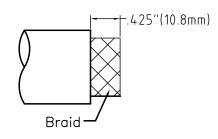
1. Cut the cable squarely and cleanly using the CCT-01 cutting tool. Use the ST-1200C-CH prep tool to remove the required length of jacket material
