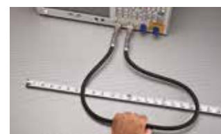
Cable is pulled off center 10" in both directions
