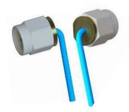
This cable utilizes Times Microwave Systems' proprietary TF4® dielectric material, eliminating the problematic non-linear phase performance of PTFE through 15-25°C and need for time-consuming extra recalibration steps or software-based phase corrections. Designed with the same diameter of the standard Semi-Rigid 047, it pairs perfectly with popular connector options:
