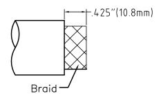
1. Cut the cable squarely and cleanly using the CCT-01 cutting tool. Use the ST-1200C prep tool to remove the required length of jacket material
