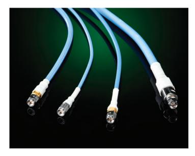
PhaseTrack PFlex cable assemblies are designed for applications demanding minimal phase change over temperature. PFlex cable assemblies are a flexible interconnect-style cable often used as a semi-rigid replacement. PFlex cables use proprietary TF4<sup>TM</sup> dielectric that does not have the abrupt shift in phase that occurs with solid or tape wrapped PTFE based products under normal room ambient conditions. PFlex cable uses the same shield construction as Times popular TFlex® cables.
