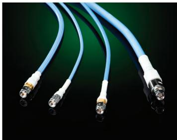
PhaseTrack® cable assemblies are designed for applications demanding minimal phase change over temperature. All PhaseTrack cables use proprietary  $TF4^{\text{\tiny TM}}$  dielectric that does not have the abrupt shift in the phase that occurs with solid or tape wrapped PTFE based products under normal room ambient—temperature conditions.
