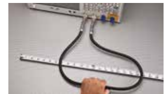
Cable is pulled off center 10" in both directions
