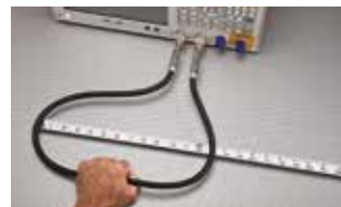
Flex Test (one full cycle)
