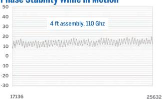
Our flex test method uses 4ft cables at 110GHz. The testing equipment calibration occurs every 8 hours. Email us at techquestions@timesmicro.com to obtain a copy of the test procedure specifications and results.
